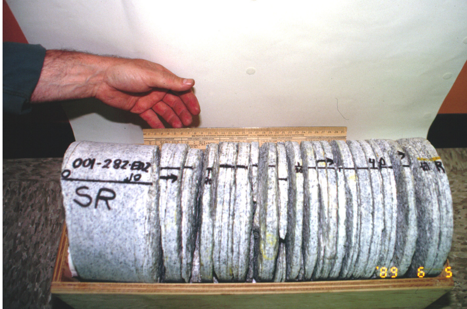
Figure 10: Disking of a 150 mm core of granite as a result of high in situ stresses.
